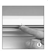
Position the cords from the right side moving rail. From the outside of the end plate, place the washer on the end of one cord into the first slot from the rear on the inside of the end plate (1). Loop the cord behind the end plate back through the second slot from the front and pull it taut to seat the washer (2).
