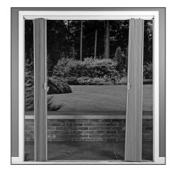
Position the left and right fabric stacks approximately 6" to 12" from their respective end plates. This provides the space needed to cord the end plates.
